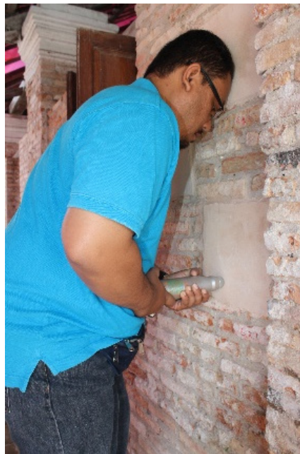
Photo 9: Conducting a test on plaster/mortar samples using the hammer rebound test Source: Kakap Mosque Conservation Project, Kedah, 2015
